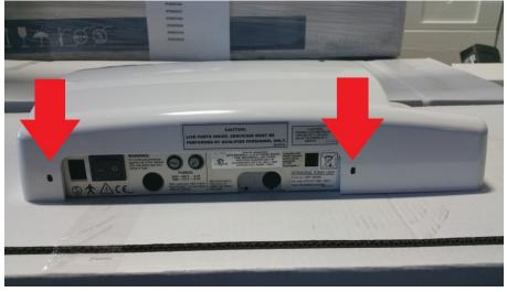
The generator housing can be detached by loosening the 2.5mm Allen screw on top of the cover next to the horizontal arm and the two 2.5mm Allen scews located on the bottom of the cover at each end of the generator board.
