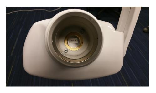
The tube head front cover can be detached by removing the two 2.5mm Allen screws located inside the cone of the tube head.
