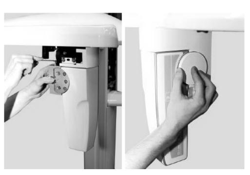
The cephalostat fixed sensor holder locking plate can be detached by loosening the 3mm Allen screw located above the axle and pushing on the axle from the outside.
