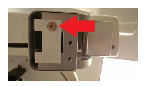
The ceph side cover can be detached be removing the 4mm Allen screw revealed when the cover plate is detached. Slide the cover horizontally towards the back of the x-ray.
