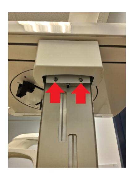
The collimator top cover box can be detached by removing the two 3mm Allen screws revealed with the collimator cover detached.
