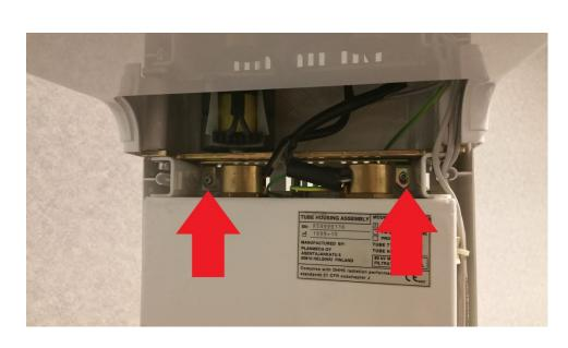
With the front tube head cover detached, the back tube head cover can detached by removing the two 3mm Allen screws located on brackets above the tubehead.
