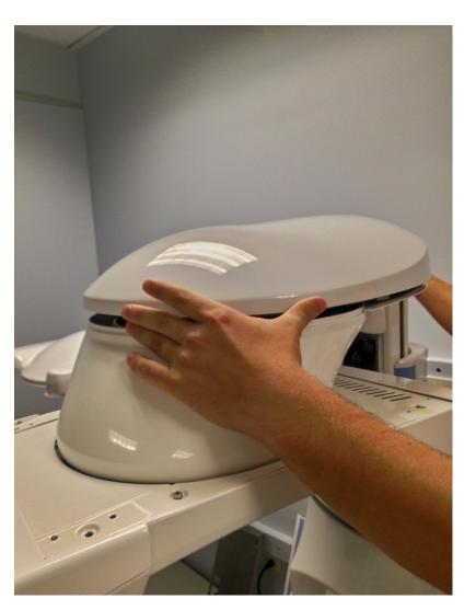
The shoulder cover can be detached by lifting up on both the front and back of the cover. The cover is held on by pressure clips and screw posts.
