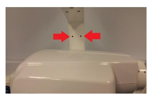
The tube head support cover assembly can be detached by loosening the two 3mm Allen screws located on the inside of the tube head support slightly above where the support frame meets the tube head support.
