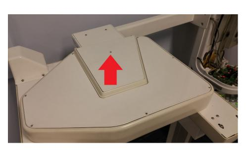
The attachment mechanism cover can be detached by removing the 2.5mm Allen screw located in the middle of the cover.
