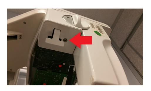
The bottom cover plate for pan connector can be detached by removing the 4mm Allen or Torx 30 screw found next to the mirror on the sensor holder.
