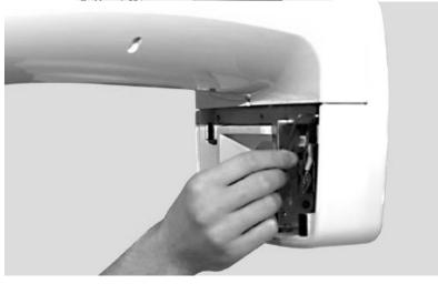
When the tube head cover plate is detached or rotated, it will reveal two 2.5mm Allen screws on the top of the connector rear cover assembly; remove these screws and the two 2.5mm Allen screws revealed inside on both sides of the sensor holder when the front connector assembly is detached.
