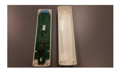
The control unit front cover and control unit back cover can be separated by pulling the rubber feet from the control unit back cover to reveal four Torx 10 screws that need to be removed.
