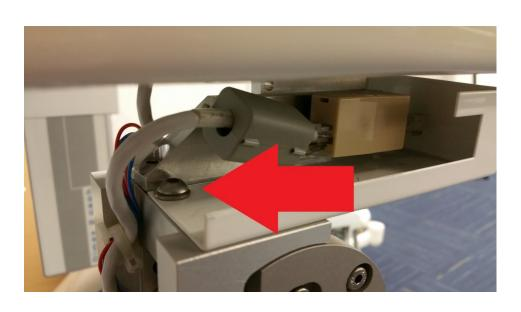
The cephalostat bottom cover can be detached by removing the 4mm Allen located near the back edge of the cover revealed once the side cover is detached. Slide the cover towards the front of the x-ray.
