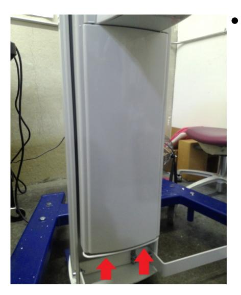
The lower front cover can be detached by pulling on the inside edge along the bottom of the cover. Since the emergency stop plate bar might be in the way, use an Allen wrench to slip behind the cover and gently pull away from the column to pop it off.
