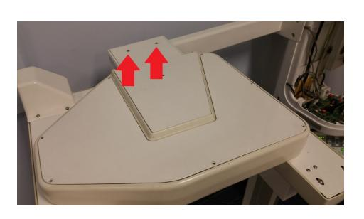
The attachment casting cover can be detached by removing the two
