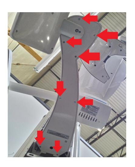
The patient support arm lower cover is detached by unscrewing (8)2.5mm Allens found under the arm along the edges of the cover.
