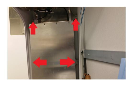
The ProMax Max sensor head back cover can be detached by removing the four 2.5mm Allen screws located on the inside of the cover revealed once the sensor head front cover is detached. Two of the screws are located towards the top while the other two are located close to the middle of the cover on the left and right sides of the sensor.
