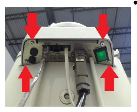
The column top cover with emergency switch can be detached by removing the four 2.5mm Allen screws located on the bottom of the input module.
