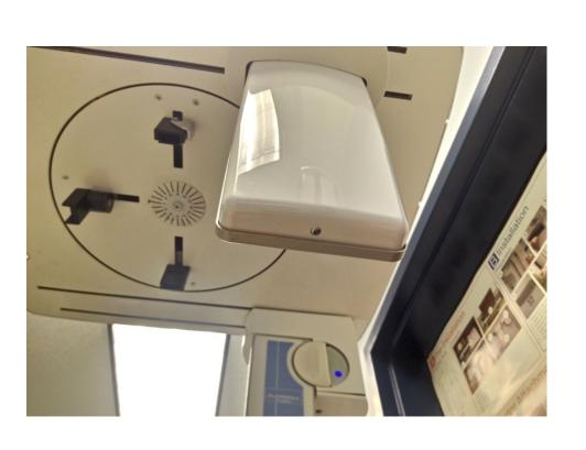
The collimator cover can be detached by removing the 2mm Allen screw on the bottom of the of the cover and pulling the cover out and down.
