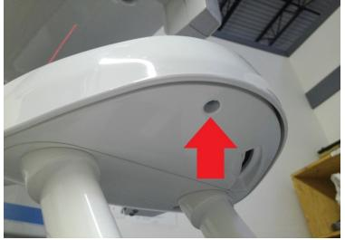
The patient support cover can be detached by removing the five 2.5mm Allen screws found under the patient support body. The front screw has a shorter length than the back four.
