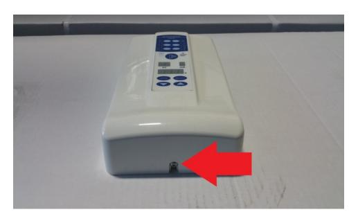
The fixed control unit housing can be detached by loosening the 2.5mm Allen screw found on the bottom of the cover.
