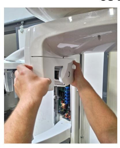
With the sensor removed, the front cover assembly can be detached by pulling on the sides of the cover towards the tube head.
