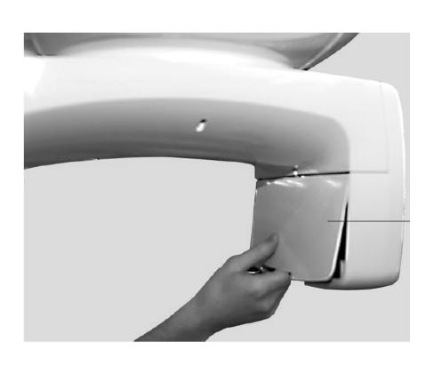
The front cover assembly can be detached by pulling on the cover. It is held on by velcro.
