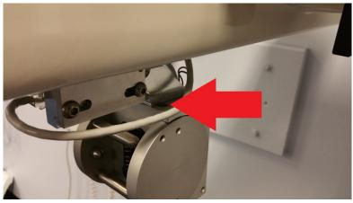
With the cephalostat bottom cover removed, the locking disc can be detached by fully loosening the two 3mm Allen screws that are recessed in holes directly above the axle rod. Once they are loose, the axle rod can be pushed and the locking disc will move freely.
