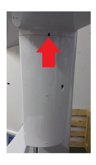
The sensor cover can be detached by loosening the 2.5mm Allen screw found at the top of the cover where it meets the carm cover and the 2.5mm Allen screw located on the bottom.
