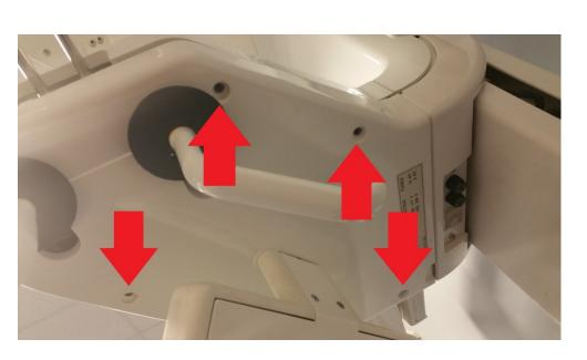
The upper cover can be detached by removing the four 3mm screws located under the table behind the GUI or touchpad.
