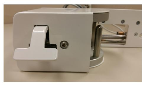
The bottom cover plate for pan connector can be detached by removing the 4mm Allen or Torx 30 screw found next to the mirror on the bottom of the sensor holder.
