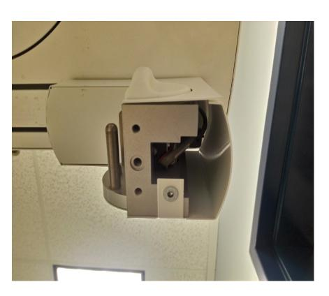
The connector back cover can be detached by removing the 4mm Allen screw revealed when the connector bottom plate is removed. Once the 4mm screw is removed, slide the cover towards the back of the machine to disengage the pressure clips found on the inside.
