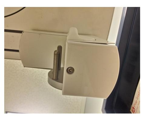
The sensor should be detached for the next 3 covers. The connector bottom plate can be detached by removing the Torx 30 screw found on the left edge of the cover.
