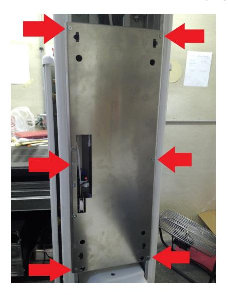
The unit may have an EMC shield under the front cover. It can be detached be removing the six 2mm Allen screws found along the sides. EMC shield for PSU2 on next page.
