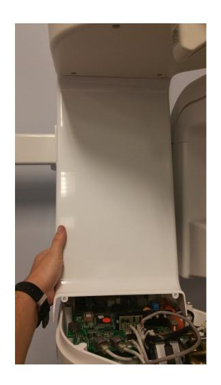
The front column carriage cover can be detached once the upper cover is detached by pulling from the base of the cover away from the column.
