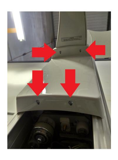
The carriage cover can be detached by removing the four 3mm Allen screws located the bottom of the cover. Two will be right below the patient support arm and two on the very bottom of the cover.
