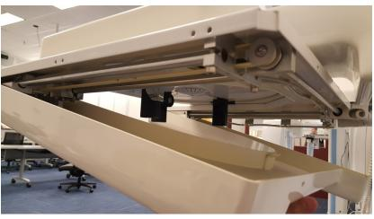
With the sensor holder and second primary collimator detached, remove the two 2.5mm Allen screws found on the back of the cover. Then lower the back half of cover and slide it away from the wall.
