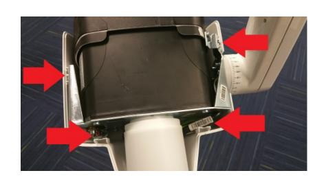
Once the upper cover assembly is off, the lower cover assembly can be detached by removing the two 2.5mm Allen screws found on either side of the tube head and the two 2.5mm Allen screws found deep inside the cover near the front of the tube head.
