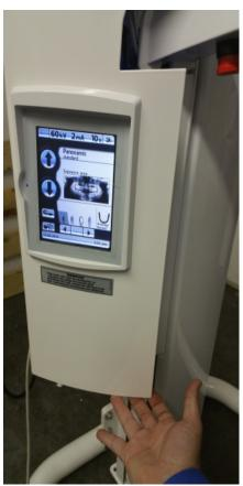
The door assembly can be opened by unscrewing the adjustment stick and pulling from the base of the door. Since the door is held closed by pressure clips and pins, it should pop out when pulled.
