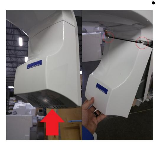
The tube head front cover can be detached by loosening the 2.5mm Allen screw located on the bottom of the cover. Once this screw is loosened, gently pull from the base while leaving the top portion still on the tube head and then down once at a 45 degree angle. The angle is to avoid breaking the two plastic arms that slide up under the c-arm cover.
