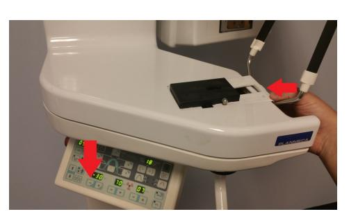
Before removing the upper cover, the dust cover must be detached. Press the mm on the touchpad or the layer left button on the GUI until the patient positioning mechanism will move no more. Push the U shaped dust cover back to reveal the lip at the front and lift it out. Then move the patient position mechanism back over the hole in the upper cover. Continued on next page.
