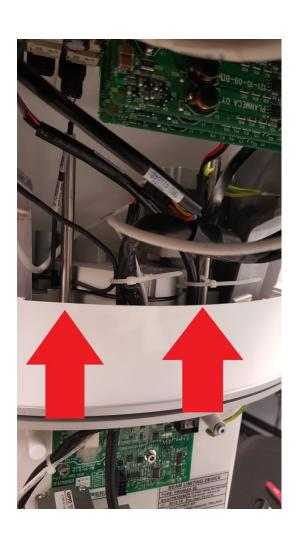
With the inner c-arm cover removed, detach the upper front tube head cover by loosening the 3mm Allen screw topped metal rods that apply pressure to the clips on the inside of the cover. These rods can be accessed by holes located directly above them.
