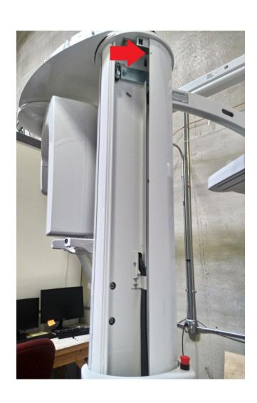
The column rear panel assemblies can be detached by raising the unit as high as it will go and then pulling gently on the inner edge of each panel near the top. The panel will pop and then pull the panel horizontally inward to unclip the top and bottom pressure brackets of the panel from the side edge of the column. More images on next slide.
