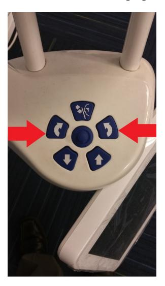
The patient support moving mechanism is in the way of removing the upper front cover on a ProMax Max/Mid/Plus. The unit should put into positioning mode by starting a full skull 3D x-ray capture sequence and the turn arrow keys on the patient position control PCB will allow the patient support moving mechanism to be moved up or down as needed.
