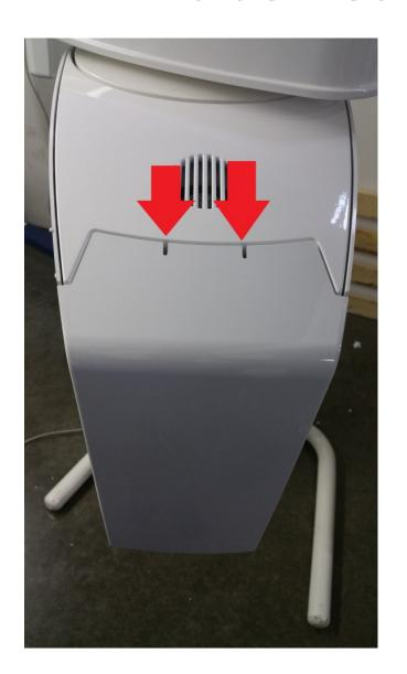
Once the tube head front cover is detached, the tube head rear cover can be detached by loosing the two 2.5 mm Allen screws located at the top of the cover.
