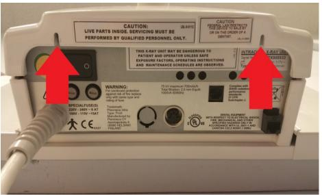
The generator cover can be detached by loosening the two 2.5mm Allen screws located on the top of the cover on either side of the horizontal arm and the two 2.5mm Allen screws found on the bottom of the cover on the left and right side of the generator PCB frame plate.
