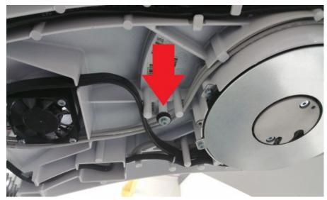
Once the tube head front cover and sensor cover are detached, the c-arm cover can be detached by gently pulling down on the cover from the sides. The c-arm cover is held on by a rubber damper located towards the center of the cover.
