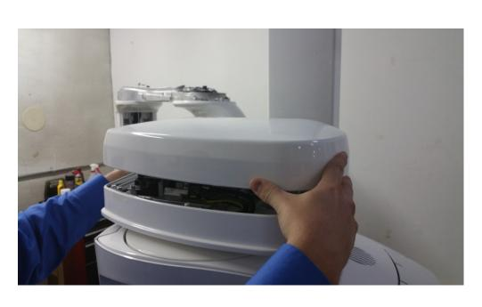
The upper arm assembly can be detached by simply lifting the cover up.
