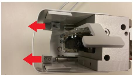
With the bottom cover plate removed, the side cover can be detached by loosening the two 2.5mm Allen screws located inside the sensor holder, near the top, screwing into square steel blocks. Once these screws are loosened the cover will slide away from the sensor horizontally.
