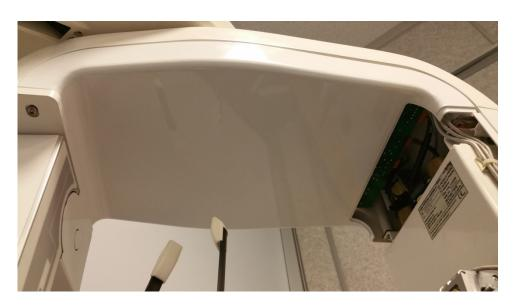
Once the front tube head cover has been removed, the inner cover can be detached by moving the edges of the inner cover by the tube head off the back tube head cover and pulling the inner cover down in front of the collimator.
