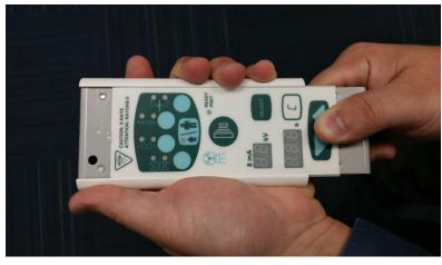
The control panel assembly can be dismantled by first removing the attachment plate on the back by removing the two 2mm Allen screws and then pulling off the upper and lower rubber covers. Next, the control panel frame can be detached by holding the cover plate while pulling up on the control panel frame.
