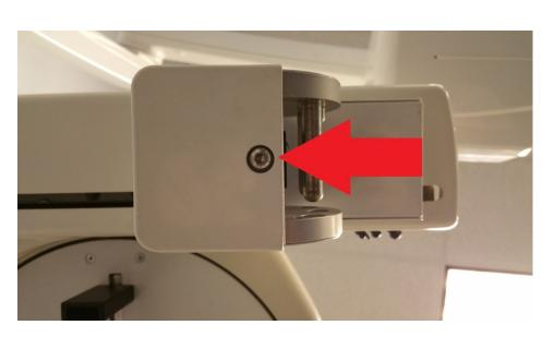
The bottom cover plate can be detached by removing the 4mm Allen or Torx 30 screw located near the edge the cover.
