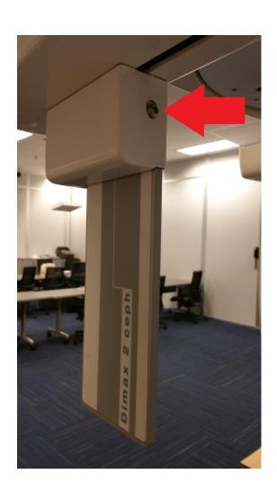
The collimator cover can be detached by removing the 4mm Allen screw located on the side of the cover.
