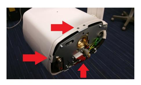
With the tube head front cover off, the tube head back cover can be detached by removing the six 2mm Allen screws found along the front edge of the cover.
